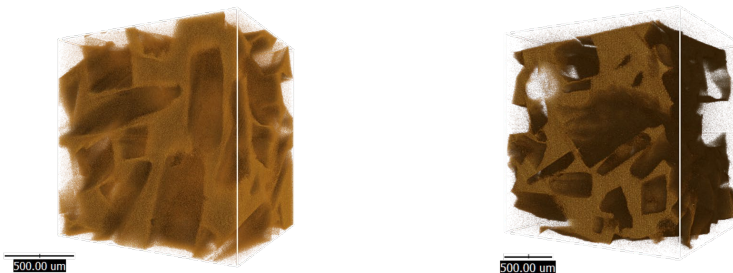
Synchrotron x-rays imaging of sponge from (left) YAG:Ce scintillation crystal (right) glass scintillator
